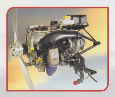
The AR682 engine has been developed to power UAVs which have limitations on propeller diameter and thereby cannot use a reduction drive. It provides 75 BHP at 6000 rpm in an ultra-compact envelope. In 1994 this power unit with all accessories successfully completed a customer-witnessed 150 hour FAR 33-type endurance test.
