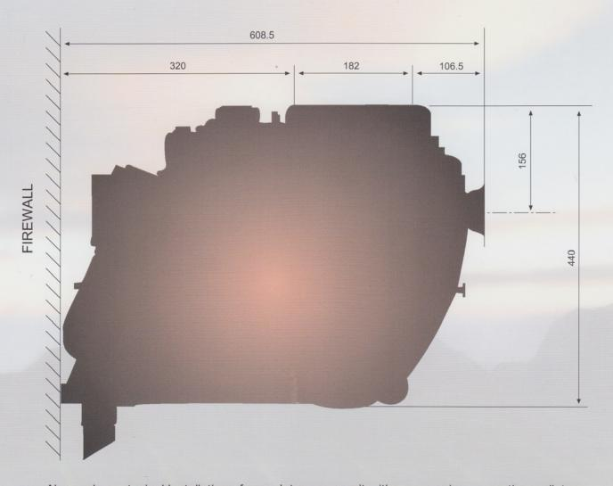
Above shows typical Installation of complete power unit with accessories, excepting radiator.
